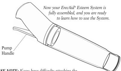
**PLEASE NOTE:** If you have difficulty attaching the pump to the cylinder, using your index finger, apply a small amount of lubricant to the outer rim of the pump. This will allow the cylinder to connect more easily. Use only a small amount of lubricant as excess can seep into the pump and cause damage.
